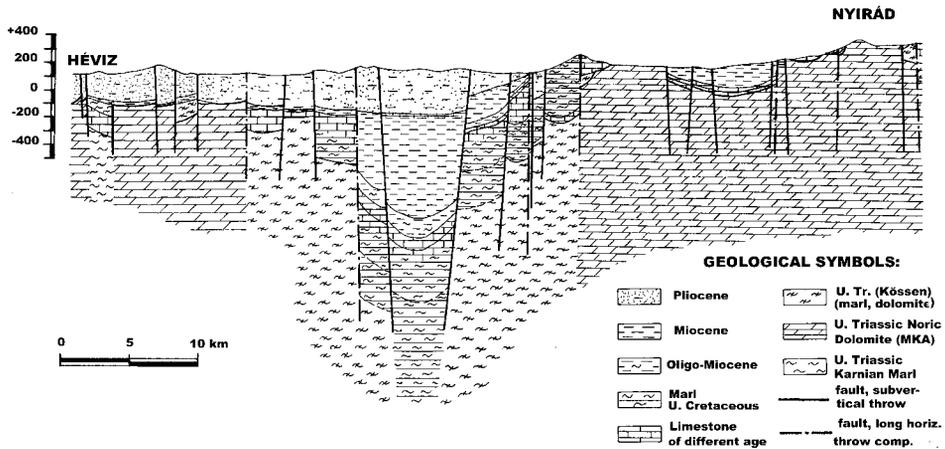
Figure 1/B Schematised geological cross section
