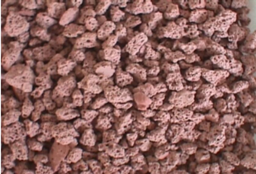
Figure 6. Granulated heavy spar bonded in foamed alumo-silicate (geopolymer)
