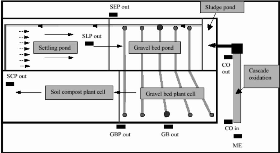
Figure 2. Schematic layout of the experimental constructed wetland at WISMUT/WISUTEC's Poehla site
