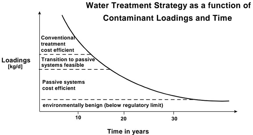
Figure 1. Typical evolution of contaminant loading and selection of cost efficient water treatment strategy
