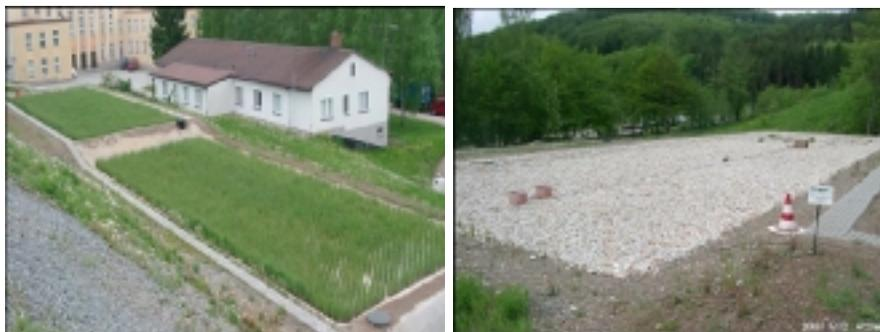
Figure 10. Experimental multi-cell wetland at WISMUT's Schlema mine site (left: plant cells, right: microbiological cell with gravel bed)
