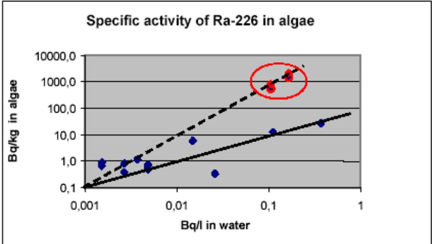
Figure 5. Sorption capacity for Radium of the macrophytic algae used in the Poehla wetland, as compared to average sorption capacity of helophytes
