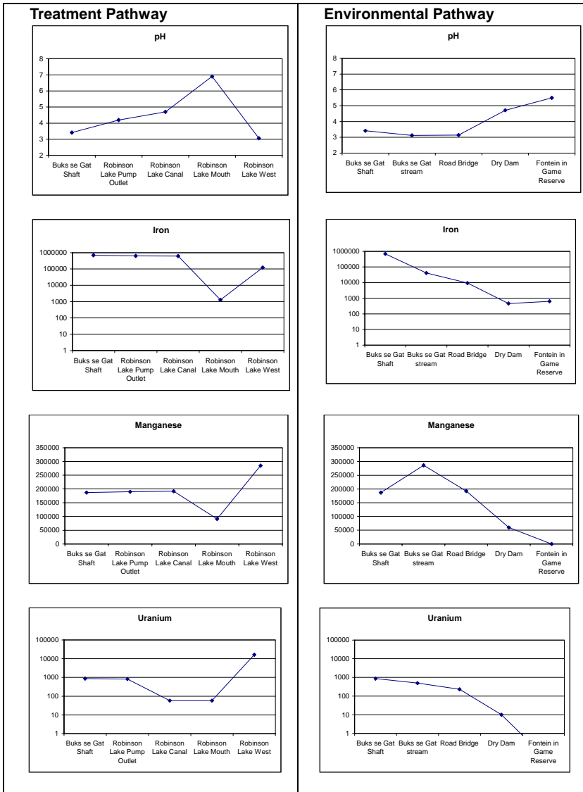
Figure 6. pH, iron manganese and uranium for the treatment and environmental pathways. (Note that iron and uranium have been plotted on a logarithmic scale.)
