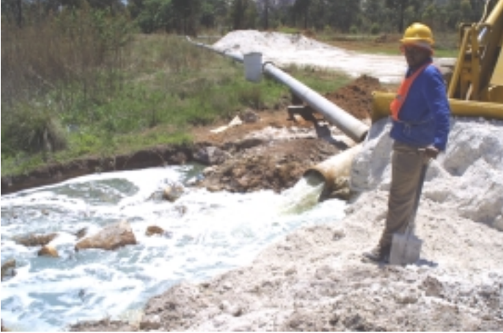
Figure 9. Worker adding lime to the water from Buks se Gat at the discharge into Robinson Lake.
