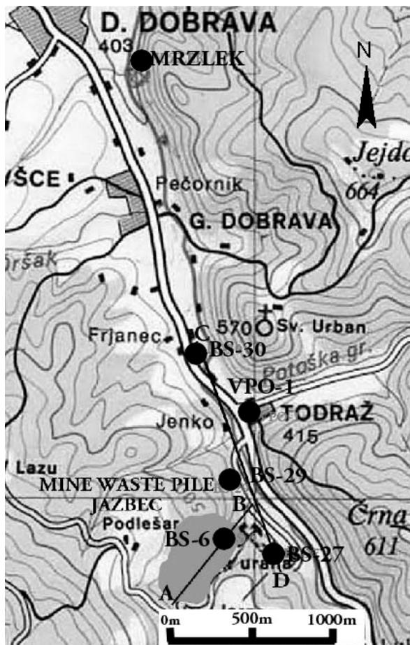
Figure 1. Location of the Jazbec mine waste pile and its piezometers.
