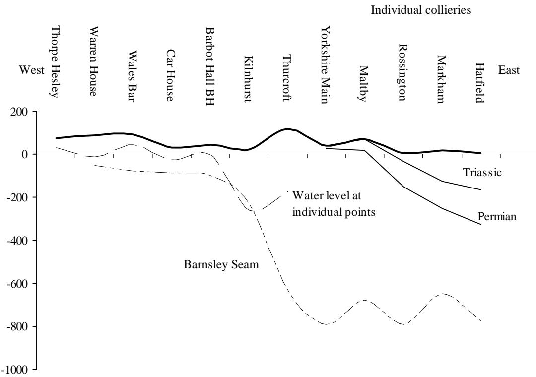
Figure 2. Present mine water levels (or last readings) at individual collieries across the coalfield from the south west to the north east. Figure 1 shows the line of cross section A to B
