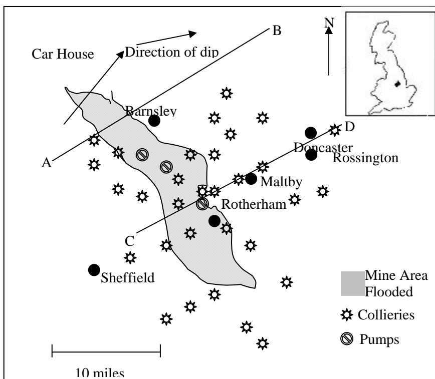
Figure 1. The South Yorkshire Coalfield with areas flooded in 1936. Cross section lines marked AB to CD are for Figures 2 and 3 (Saul 1936).
