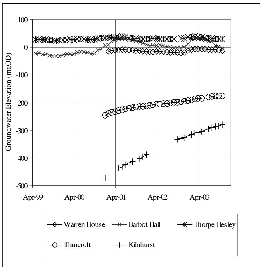
Figure 5. Mine water recovery at selected collieries over time shown in Figure 3
