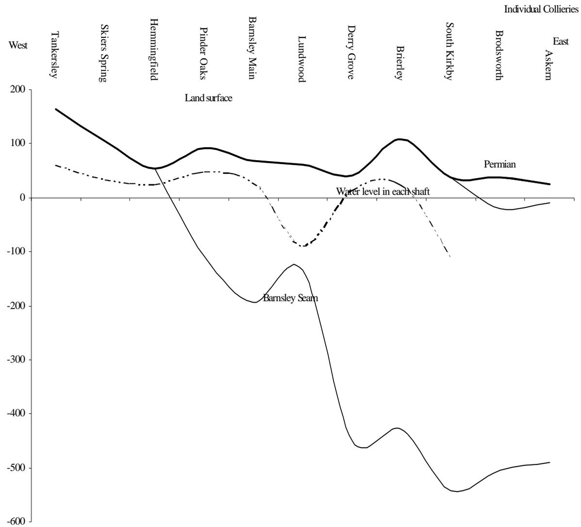
Figure 3. Present mine water levels (or last readings) at individual collieries across the coalfield from the south west to the north east. Figure 1 shows the line of cross section C to D
