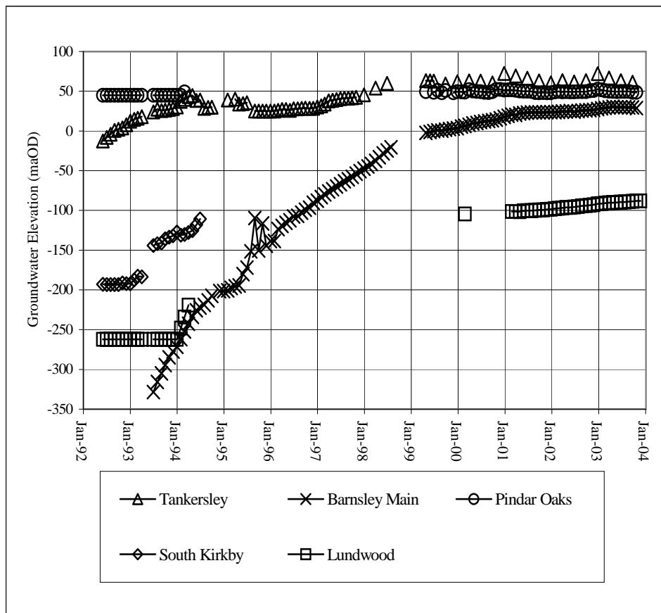
Figure 4. Mine water recovery at selected collieries over time shown in Figure 2
