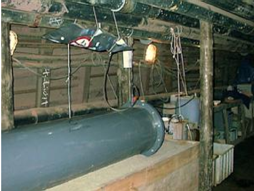
Fig. 5. View of underground column tests to find and check suitable reactive materials to treat flooding water
