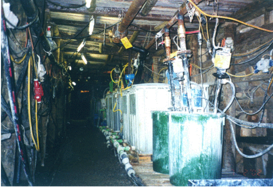
Fig. 4. View of the apparatus used for the preparation of 100,000 m 3 BaSO 4 forming solution
