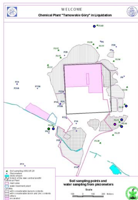
fig1. Map of the Tar-nowskie Góry megasite and relevant concentrations of heavy metals. Blue spheres indicate Zn concentrations above 500 µg/l, green spheres Cu concentrations above 100 µg/l, and purple spheres As concentrations above 40 µg/l.
