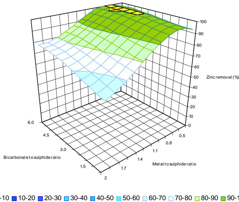
**Fig. 1.** Response surface, modelling zinc precipitation by a combination of sulphide and bicarbonate. Note: Y-axis (M:S ratio) scale reversed to allow better visualisation of the surface.
