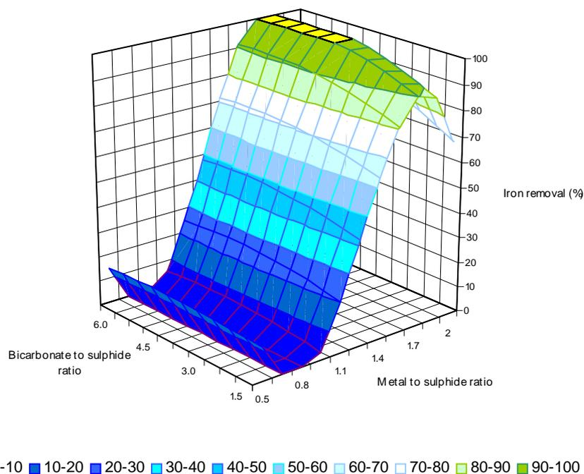
**Fig. 2.** Response surface, modelling iron precipitation by a combination of sulphide and bicarbonate
