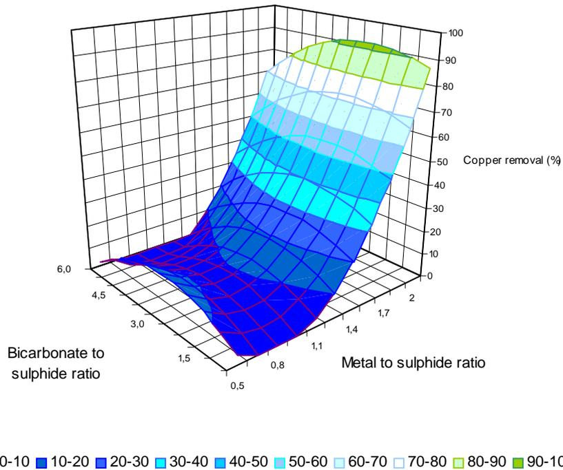
**Fig. 3.** Response surface, modelling copper precipitation by a combination of sulphide and bicarbonate
