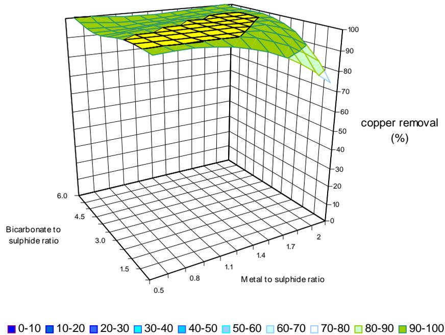
**Fig. 4.** Response surface obtained using data points generated using the aqueous species modelling software MinteqA2. The data points were obtained by modelling the 32 conditions tested experimentally
