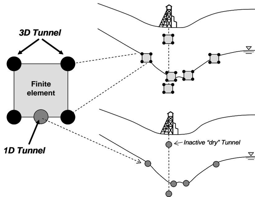
**Fig. 1.** Schematic of 3D and 1D seepage face boundary approach for regional models, showing concept that at large scales, 1D tunnels produce similar results to 3D-tunnels.
