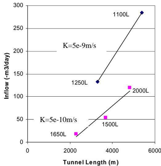
**Fig. 2.** Graph showing relationship between cumulative 1D tunnel length and inflow for two bedrock conductivity zones
