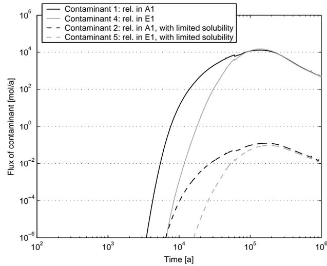
**Fig. 4.** Contaminant flux from the overlying rock into a near-surface aquifer for contaminants 1 and 2 (released from cavern A1) and contaminant 4 and 5 (released from cavern E1)
