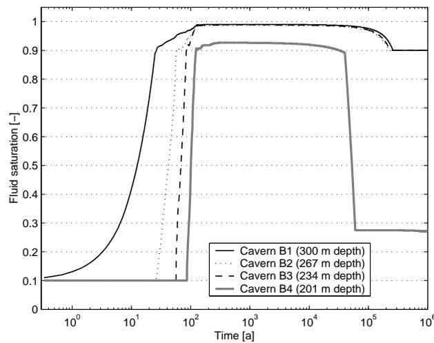
**Fig. 2.** Temporal evolution of the water saturation in the mine, exemplified with one cavern representing one mine level each (caverns B1 to B4)
