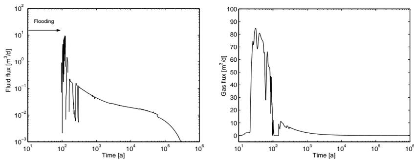
**Fig. 5.** Fluid flux and gas flux from the mine into the overlying rock via the connecting pathway
