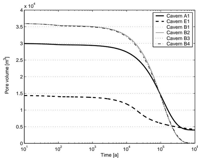
**Fig. 3.** Temporal evolution of the pore space in the mine, exemplified with the two caverns containing waste materials (cavern A1 and cavern E1) and one cavern representing one mine level each (caverns B1 to B4 = overlapping curves)
