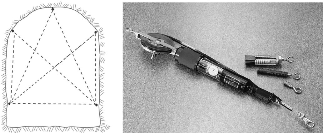
Figure 12: Tape extensometer
