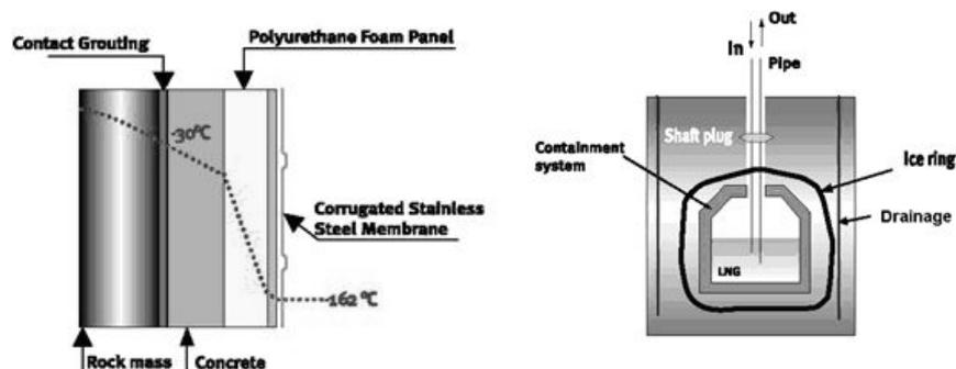
**Figure 3: Schematic principle of containment for LNG storage cavern**
