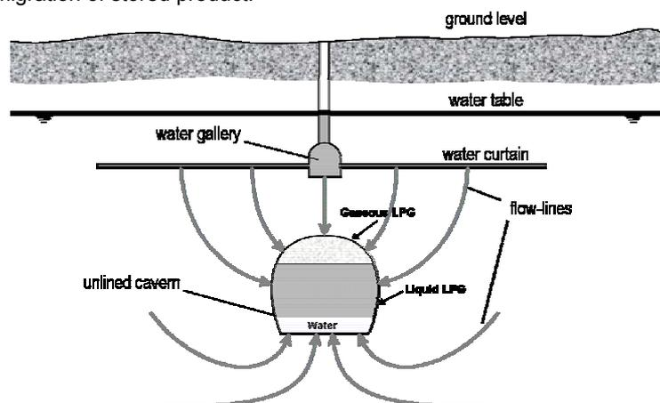
Figure 1: Schematic principle of containment criteria for LPG storage cavern
