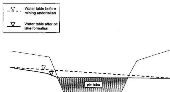
**Figure 4: Pre-extraction and post-pit lake formation water table profiles around a pit lake in flooded sand and gravel workings (after Younger *et al.*, 2002)**
