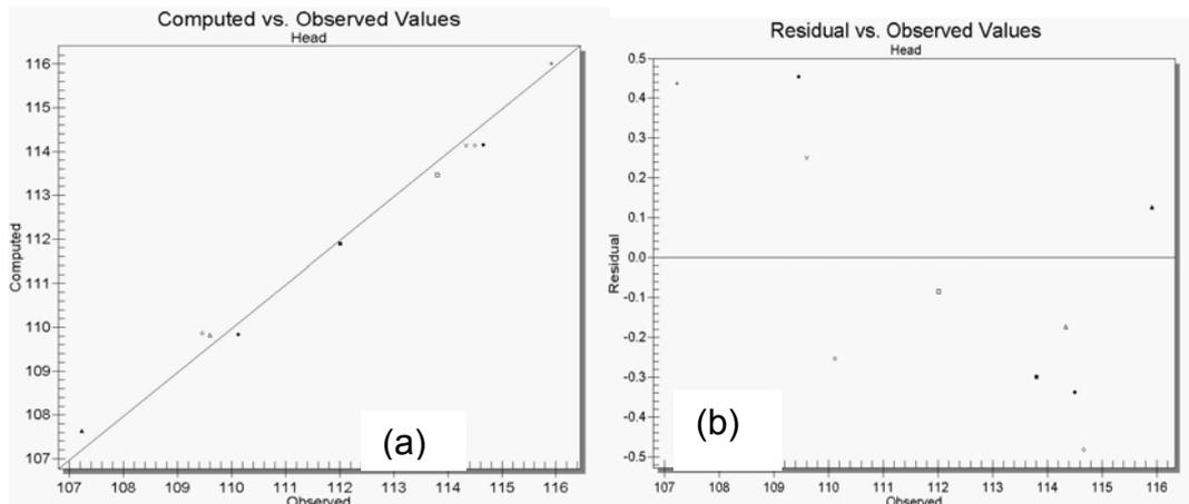
Figure 2: Steady state calibration showing (a) computed versus observed groundwater heads (mAOD) and (b) residual versus observed groundwater heads (mAOD)
