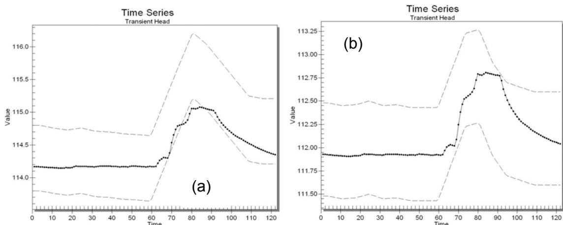
**Figure 3: Time series for groundwater heads in borehole 5 (a) and borehole 9 (b) (mAOD) during transient simulation, showing calibration targets**
