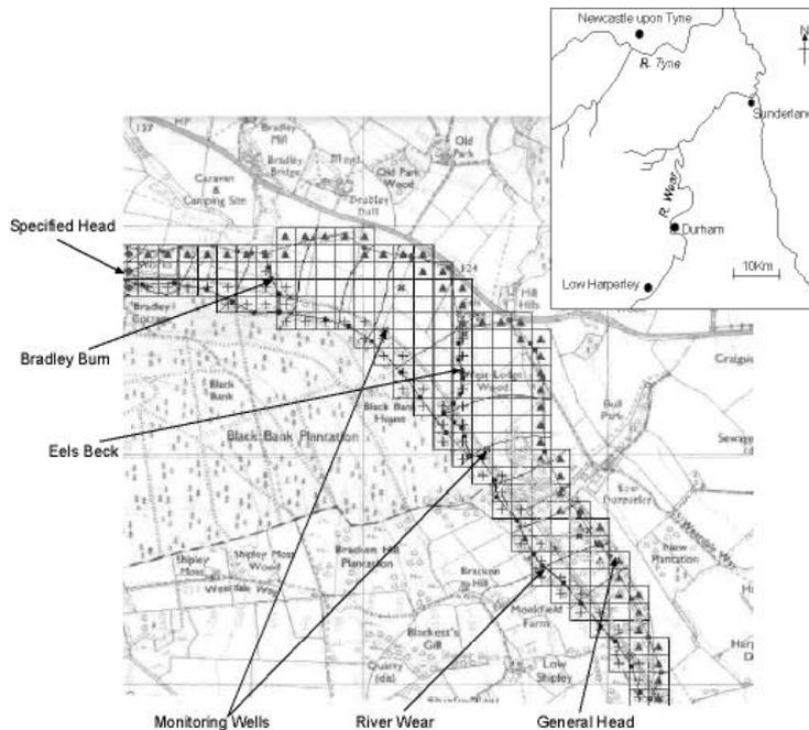
**Figure 1: Conceptual model showing location of Low Harperley, boundary conditions, rivers and monitoring wells**
