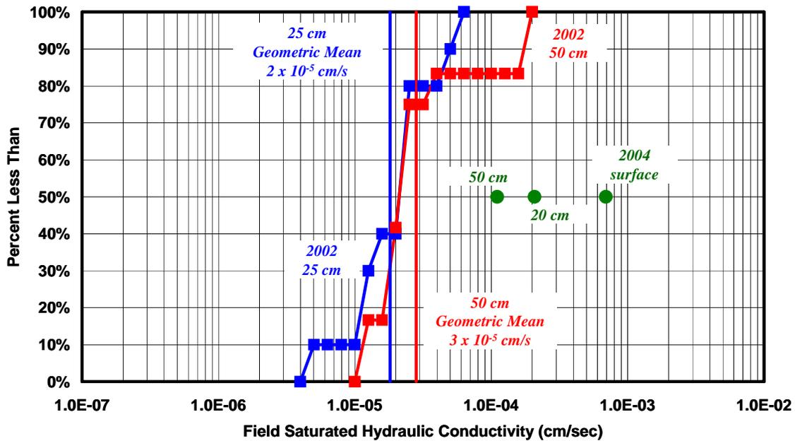
Figure 6. Field saturated hydraulic conductivity measurements at PTMS #2.
