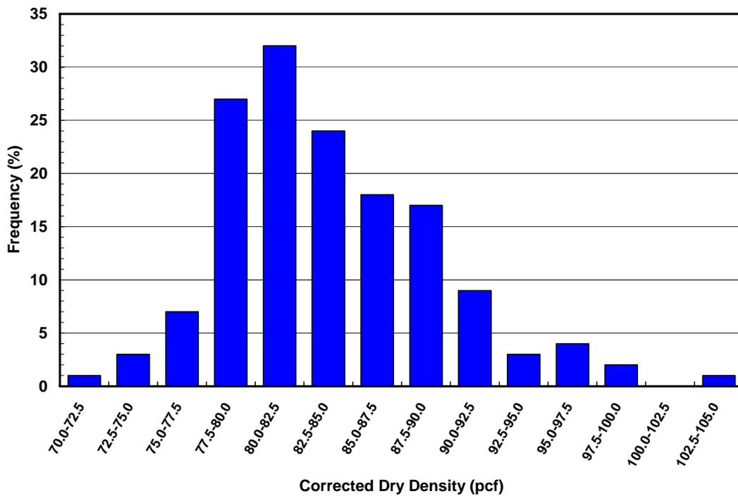
Figure 3. Frequency distribution of corrected *in situ* density conditions for the near surface cover material.
