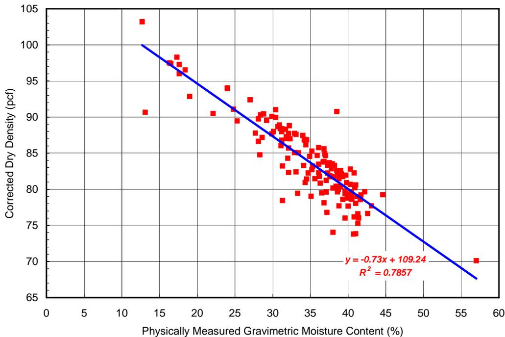
Figure 4. Relationship between corrected dry density and physically measured gravimetric moisture content for the near surface tailings dam cover material.
