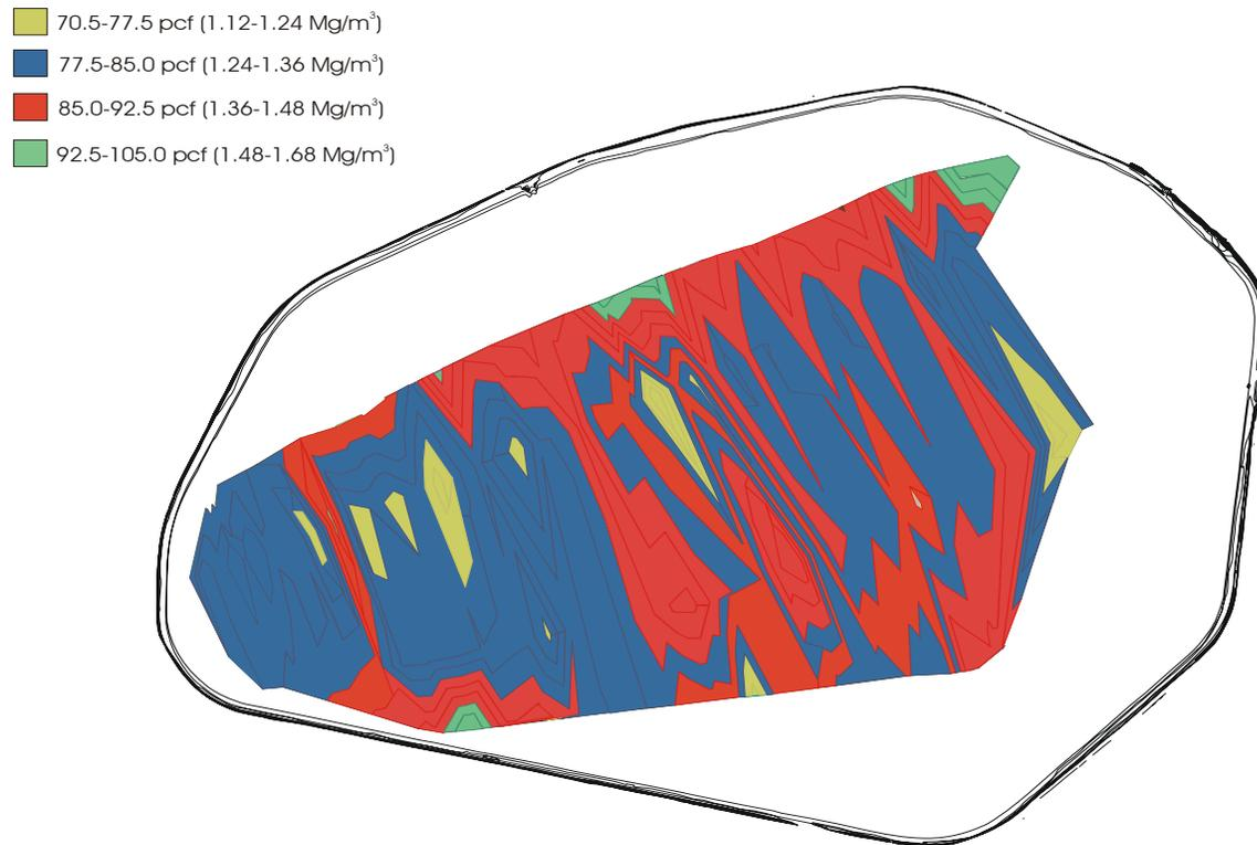
Figure 5. Tailings dam cover system plan view of the spatial distribution of corrected *in situ* density conditions for the near surface cover material.
