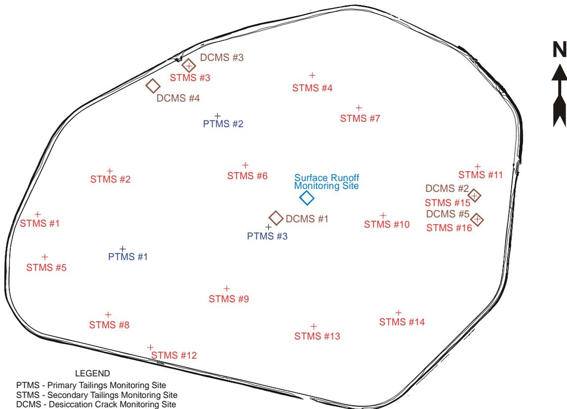
Figure 1. Schematic showing location of the tailings dam cover system performance monitoring system.
