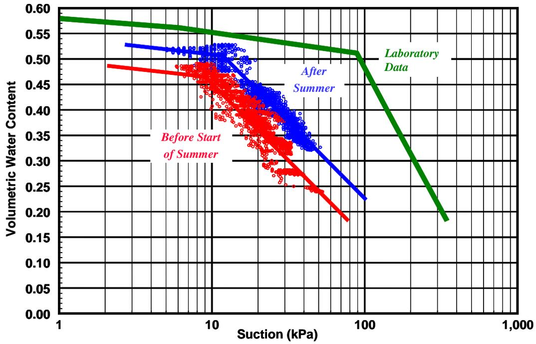
Figure 7. Field and laboratory moisture retention curves at a depth of 20 cm at PTMS #2.
