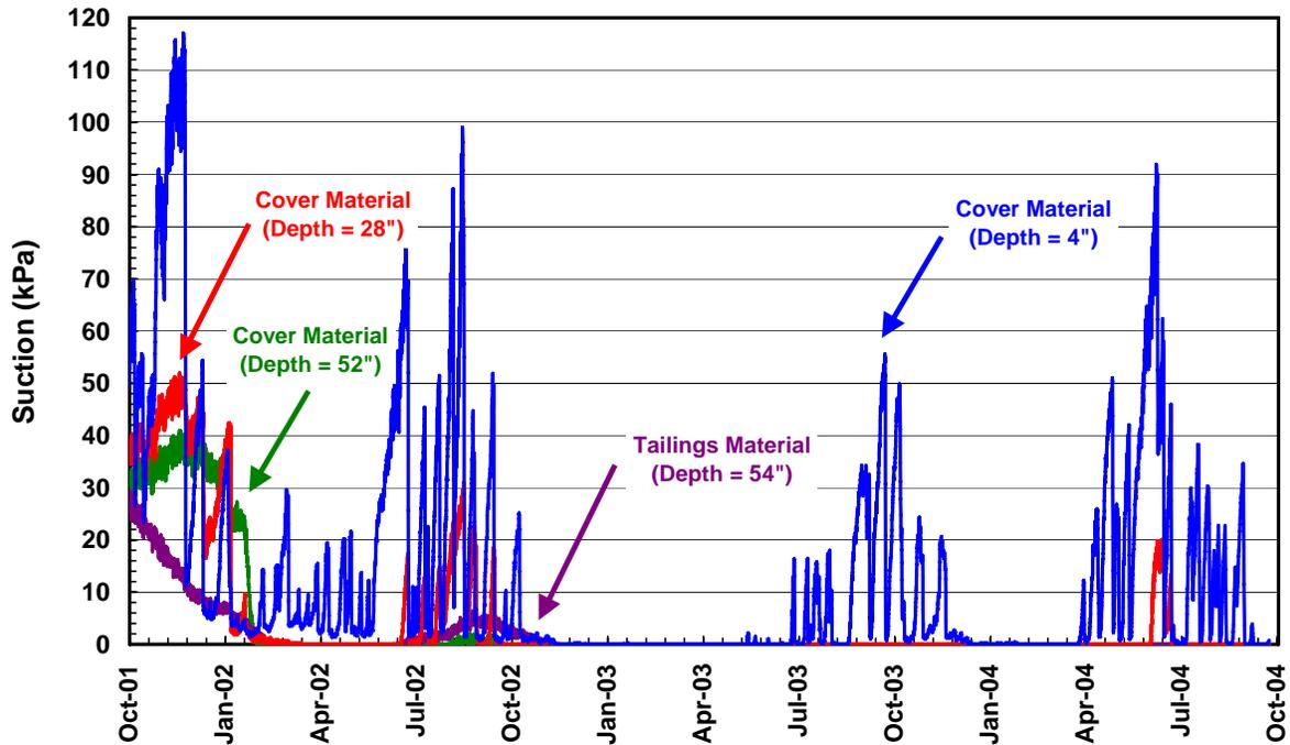
Figure 9. Field matric suction as a function of time for the sensors installed in the cover and tailings material at PTMS #1.
