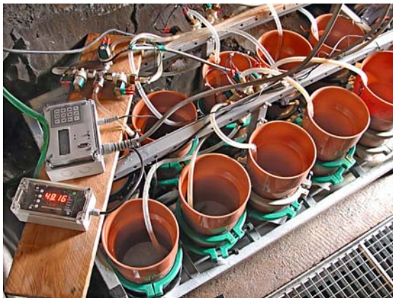
Figure 2. Sampling equipment (Multiple Filter Storage Tool: MeFiSTo) for a multi-tracer test with microspheres including flow-meter and electronic control device.
