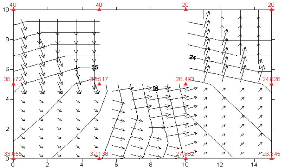
Figure 5. The flow direction vectors, hydraulic head values at nodes (indicated by small solid triangles) and hydraulic head contour lines for the simplified model shown in Figure 4.
