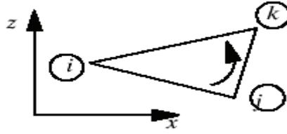
**Figure 3. Each triangular element has three nodes  $i, j$  and  $k$  arranged in counter-clockwise direction.**
