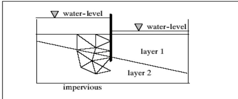
Figure 2. The groundwater model discretised by triangular finite elements.
