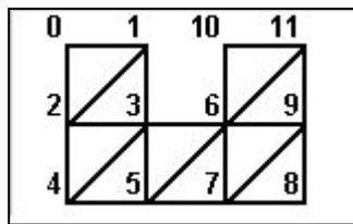
Figure 4. A simplified model with nodes numbered from 0 to 11 in the triangular element grid.
