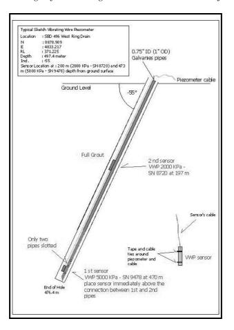
Figure 11 Typical design of a Vibrating Wire Piezometer at Batu Hijau in a core hole
