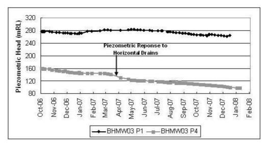
Figure 13 Data from Vibrating Wire Piezometer BHMW03 at Batu Hijau
