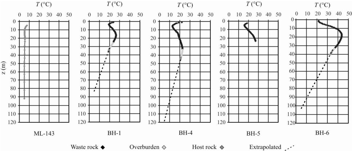
Temperature measurements made during the 1900's indicated that the dump internal temperature ranged from 20 to 65 °C (Choquette and Gélinas 1996; Lefebvre et al. 2001a). The temperature has since been slowly decreasing. Additional temperature measurements were performed in 2007 at the
