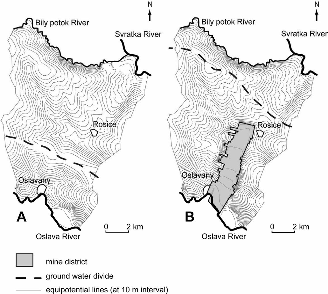
independent flow domains. As a result of dewatering by drainage gallery and hydraulic interconnection of mines, the ground water divide has moved some 5-7 km to the North. Compared to original period preceding the mining activities, the catchment area of the Oslava River has increased (fig. 3). This is in good agreement with the observations in the field, where quite large infiltration of
