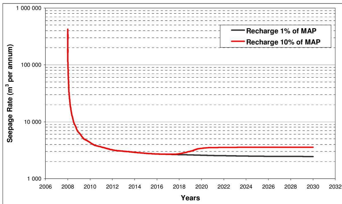
The saturated and unsaturated seepage curves were combined to reflect the changeover from wet to dry deposition.
