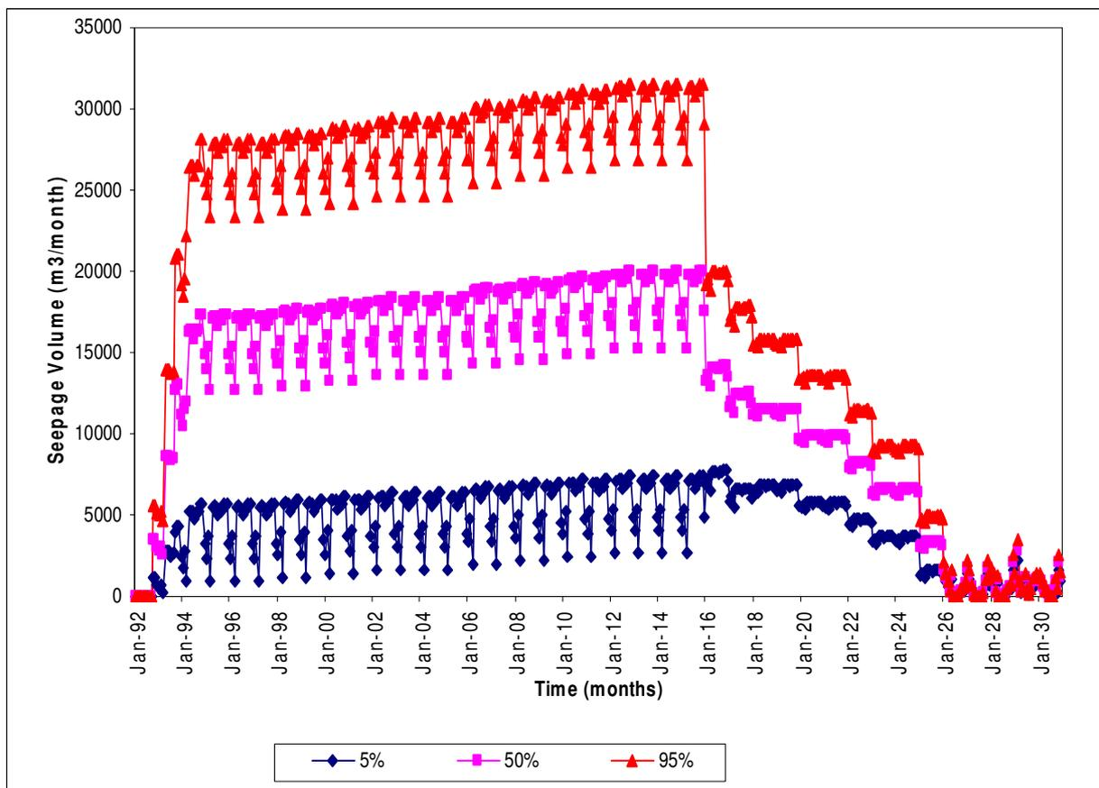
Seepage from the dry deposition of coal fines was assessed by unsaturated flow modelling.
