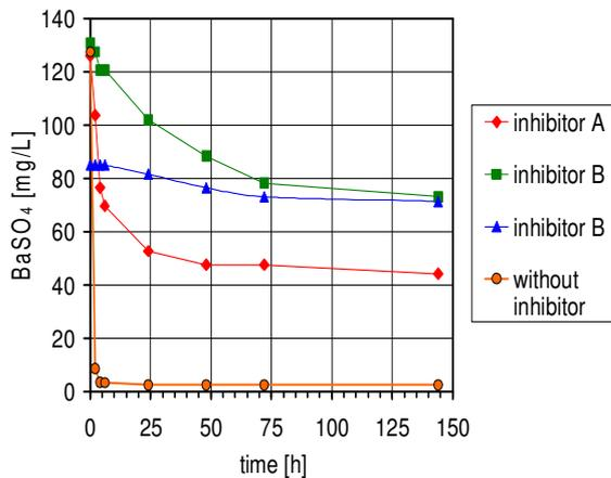
**Figure 5** Outflow concentrations in column experiments to characterise the action of BaSO<sub>4</sub> solutions
