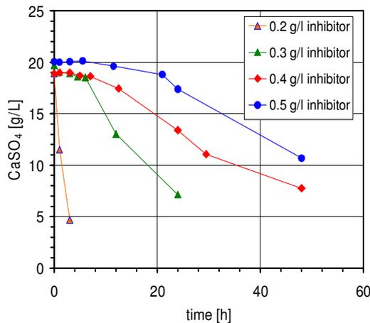
**Figure 3** CaSO<sub>4</sub> outflow concentrations and k<sub>f</sub> values during treatment a sand column with gypsum forming solutions
