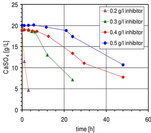
**Figure 3** CaSO<sub>4</sub> outflow concentrations and  $k_f$  values during treatment a sand column with gypsum forming solutions
