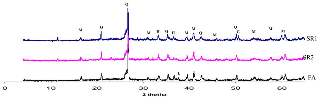
Figure 2. XRD spectra of FA, solid residues (SR1 and SR2) after treatment of CMW with FA.
