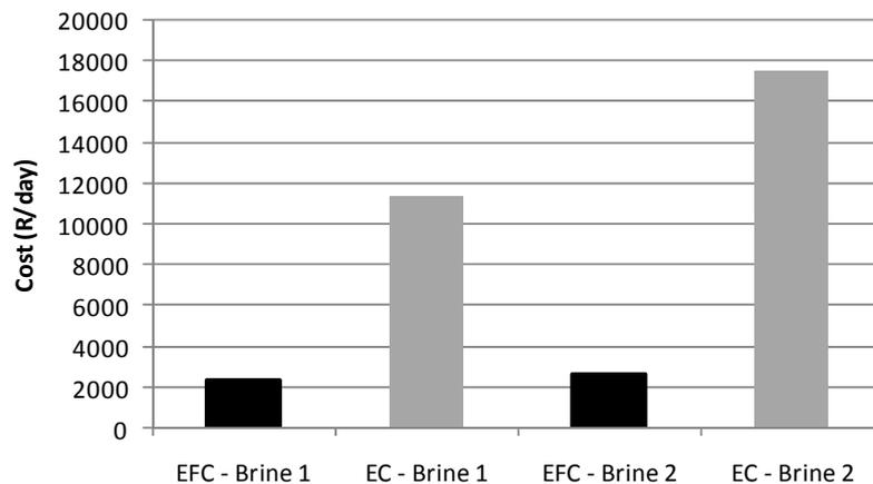
Figure 4. Comparison of daily operating costs for treating Brines 1 and 2 with EFC and multi-stage evaporation (Basis = 100m<sup>3</sup>/day of brine)
