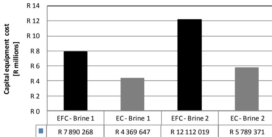
Figure 5. Comparison of the capital cost of equipment for Brines 1 and 2 for EFC and EC (Basis = 100m<sup>3</sup>/day of brine)
