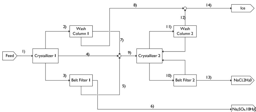
Figure 3. Basic sequential EFC process flow sheet for Brines 1 and 2
