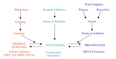
Figure 4. Schematic of the Contributions to Solution, Precipitates and Mineral Surfaces (Smart, Skinner and Levay, 1999)
