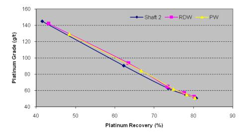
Figure 5. Effects of Underground Water (Shaft 2), Return Dam Water (RDW) and Process Water on Platinum Flotation at Amandelbult
