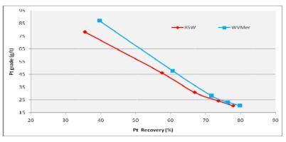
Figure 6. Effects of Rustenburg Treated Sewage Effluent (RSW) and Waterval Merensky Process Water on Platinum Flotation at Rustenburg
