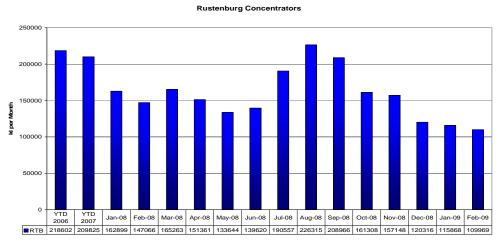
Figure 7. Potable Water Consumption Before and After Replacement with Treated Sewage Effluent for Gland Service Water
