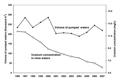
Figure 1. Amount of mine water and uranium concentration in mine waters drained from the flooded Olší – Drahonín deposit to the purification plant
