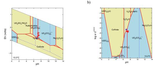
Figure 4. Redox-pH (a) and activity-pH (b) stability diagrams for uranium in mine water at 13.2 °C and component concentrations determined analytically. Blue stars – conditions in mine water from borehole at depth 170 and 210 m below surface, red circles – mine water discharged from mine at dewatering adit.
