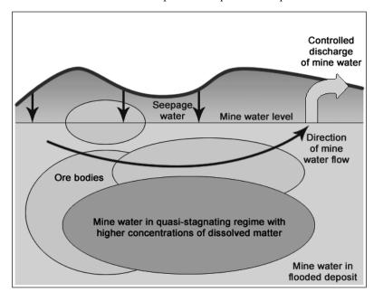
Figure 2. Diagram of expected distribution of mine waters in the flooded mine under closure
