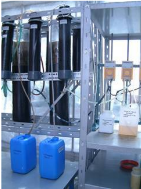
Figure 2. experimental set-up – left: columns (volume 4.8 l), right: box (volume 90 l)
