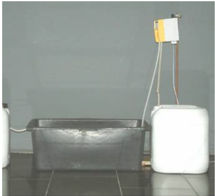
Figure 2. experimental set-up – left: columns (volume 4.8 l), right: box (volume 90 l)
