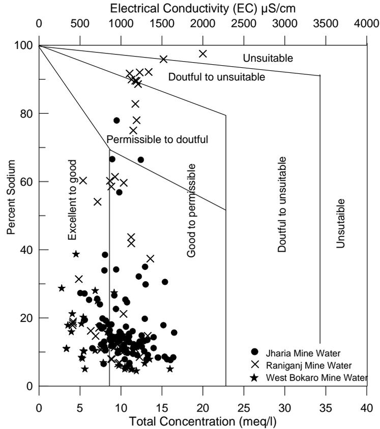
Fig. 3. Wilcox diagram relating electrical conductivity (EC) and sodium percent (%Na)
