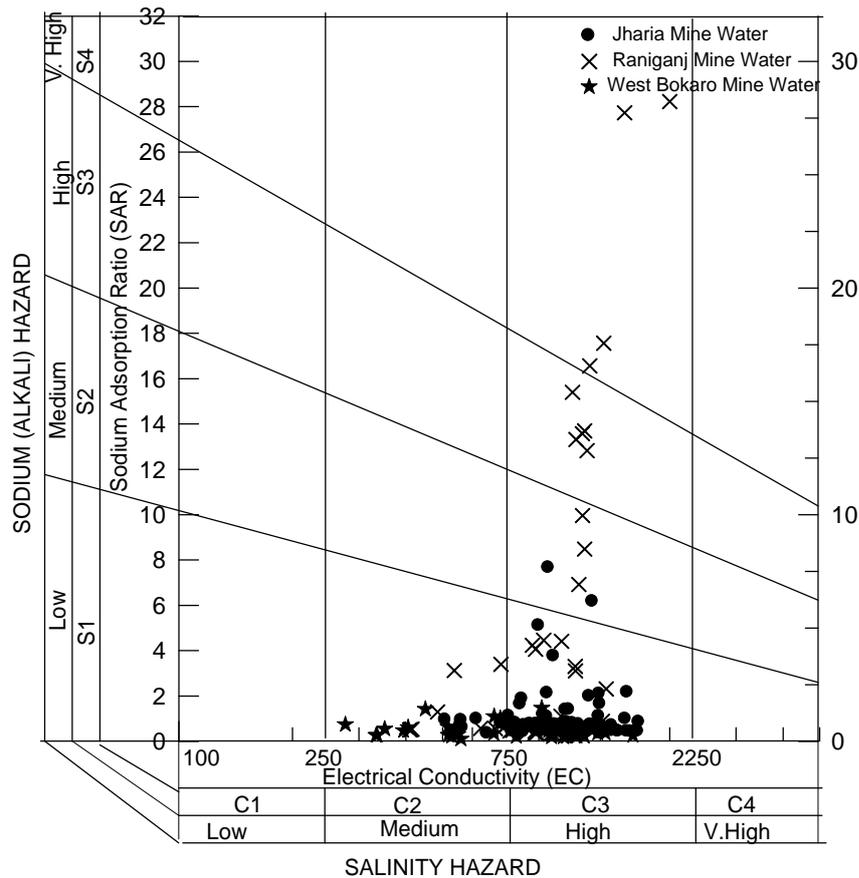
Fig. 4. The plot of data on the US salinity diagram (After Richards 1954)
