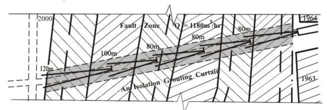
Fig.2 Schematic arrangement of grouting boreholes for ground treatment of water-bearing fault zones at crosscut No 6 of Radyanska coal Mine, Ukraine
