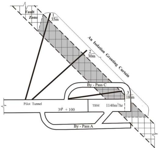
Fig.3 Arrangement of grouting boreholes for elimination sudden inrush of water into Pin Lin Pilot Tunnel
