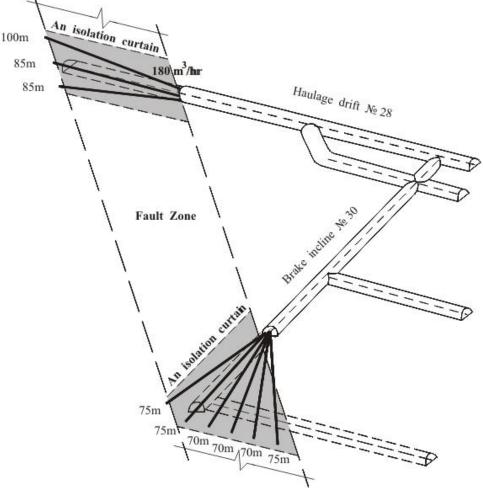
Fig.1 Elimination of sudden inrush of water in horizontal and inclined drifts of the Kievskaya coal Mine in Ukraine
