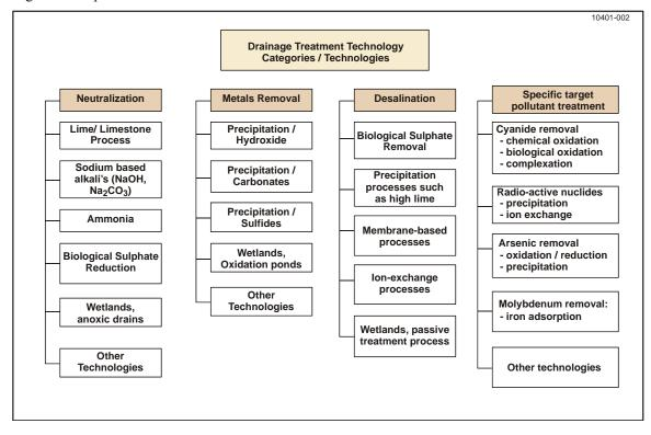
Figure 5. Generic Range of Drainage Treatment Technologies
