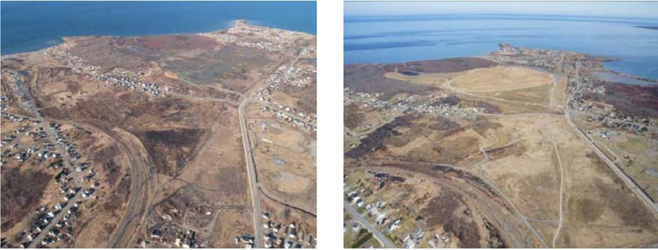
*Figures 2 and 3 Photo to left represents waste rock pile prior to remediation (2007). Photo to right represents waste rock pile post remediation (2010)*
