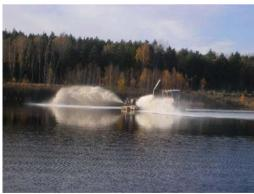
Figure 1 Spreading boat in action: A slurry of  $CaCO_3$  and lake water is prepared on the boat and distributed up to 25 meters to each side of the boat. The boat distributes up to 250 tons  $CaCO_3$  per day
