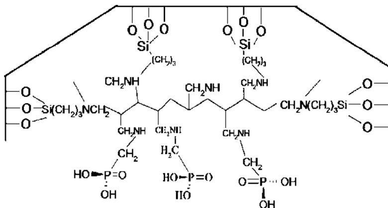
Figure 1 Structure of the BPAP silica polyamine composite
