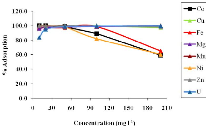
**Figure 3** Metal ion adsorption dependence on concentration
