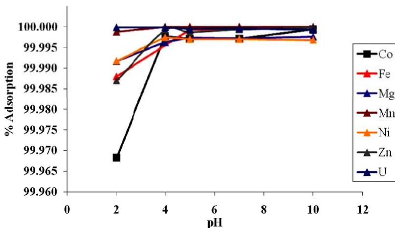
Figure 2 Metal ion adsorption dependence on pH
