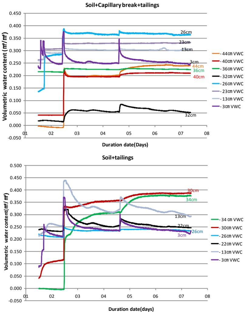
Figure 1 Water content sensor response in a tailings to suction(simulated bottom) of distilled water(a:3 layers, b:2 layers)
