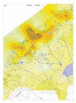
Figure 3 Groundwater flowing in the forefield of the ČSA mine – eastern part
