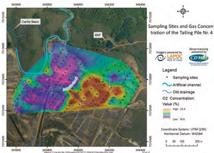
Figure 2 Gas concentration map for O<sub>2</sub> at WRP4.
