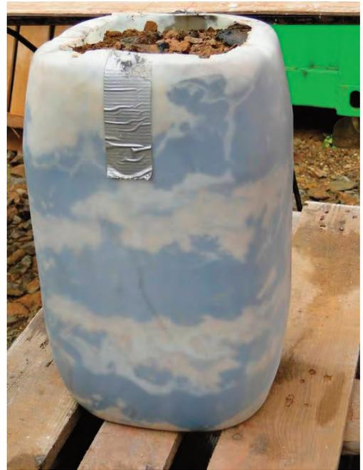
Figure 3 One of the 25 L pilot trials after injection. Different layers with mine waste and alkaline amendment can be seen.
