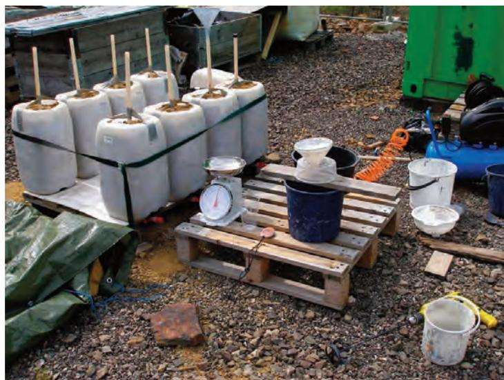
**Figure 1** Small pilot trials (25 L) with the plastic pipes for injection.
