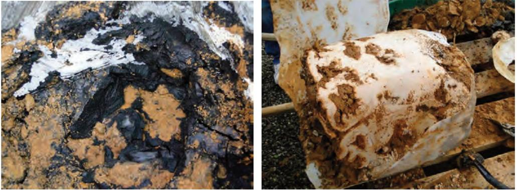
*Figure 4* Deconstruction of 25 L pilot trials. Injection with green liquor dregs (left) indicate that all voids have been filled and that impermeable layers have been formed. Mine waste injected with lime kiln dust (right) has formed a solid unit with very low permeability.
