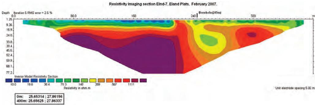
Figure 2 Geophysical profile 7, shows where high-wall ends and boreholes was positioned.
