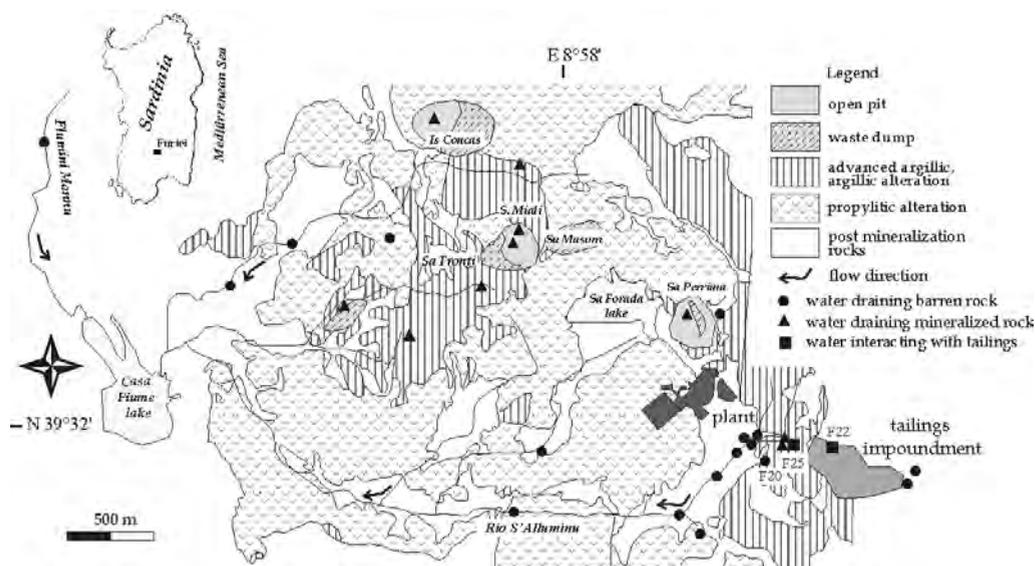
**Figure 1** Schematic map showing the gold mine area at Furtei (Sardinia, Italy), main alteration facies in Tertiary volcanic rocks and the location of water samples.
