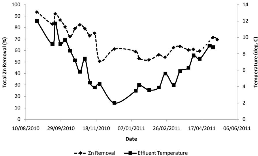
Figure 2 Percentage total zinc removal and effluent temperature in pilot-scale system.
