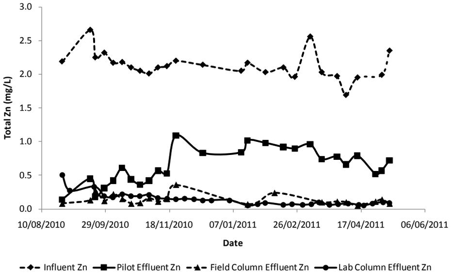
**Figure 1** Influent and effluent total zinc concentrations in the lab column, field column and pilot-scale system.
