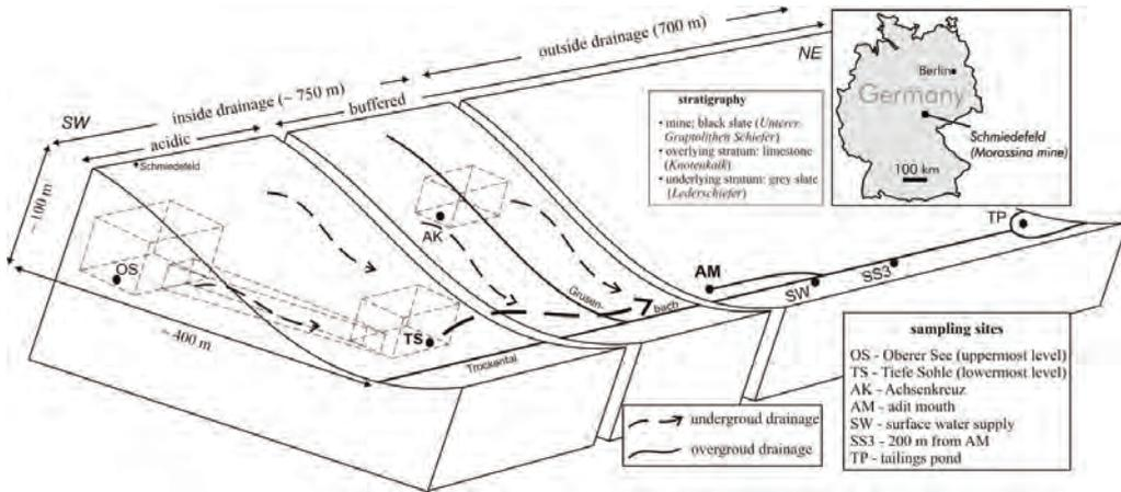
Figure 1 Drainage system of the Morassina mine in Schmiedefeld (Thuringia, Germany) (not to scale).
