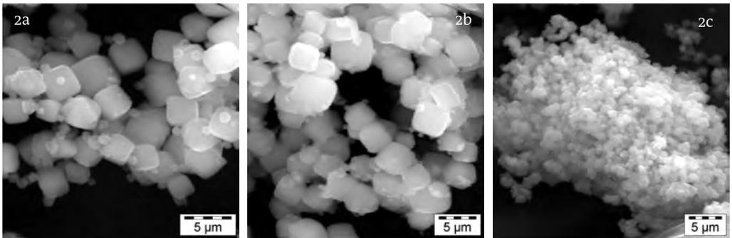
**Figure 5** SEM images of zeolite A synthesized using different solvents 2a) pure water, 2b) CNW and 2c) AMD with sonication at 100 °C for one hour using a clear synthesis solution.
