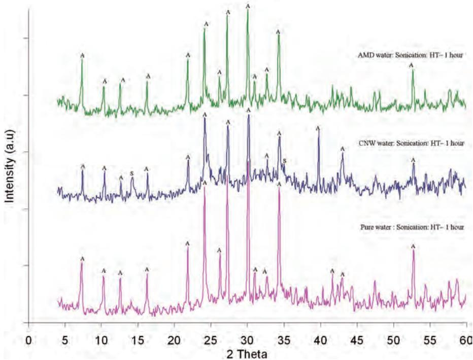
Figure 3 XRD comparison of zeolite samples synthesized using UP water, CNW and AMD mine waters synthesized from the raw fly ash slurry.
