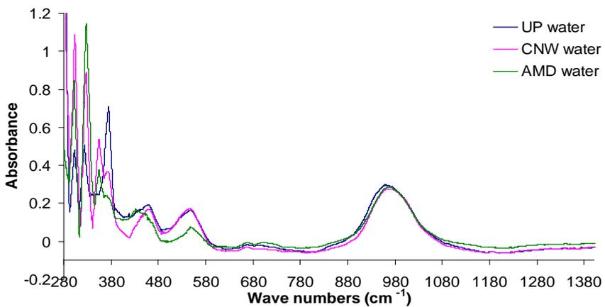
**Figure 6** Comparison of spectra of zeolite synthesized using different synthesis solvents (UP water, CNW mine water and AMD mine water).
