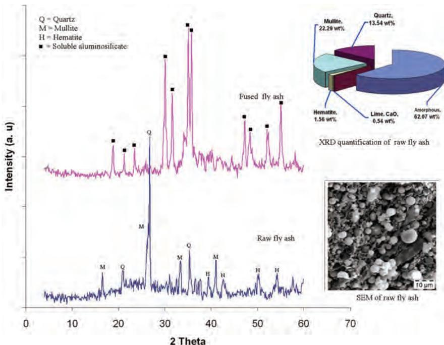
*Figure 1 XRD patterns of raw and fused fly ash: Inset: Quantitative XRD analysis and SEM of raw fly ash.*
