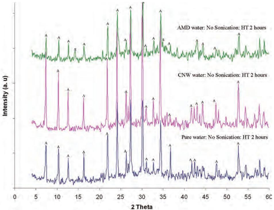
Figure 2 XRD patterns of zeolites synthesized by substitution of ultra pure water with acidic (AMD) and circumneutral (CNW) mine water.
