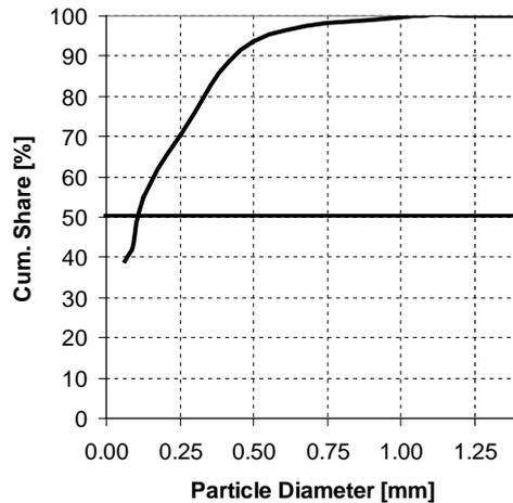
Figure 3 Particle size distribution of limestone that is used for the overburden buffering at Garzweiler.
