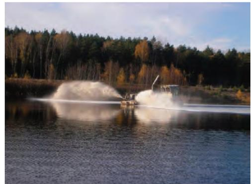
**Figure 5** Spreading boat in action: A slurry of CaCO<sub>3</sub> and lake water is prepared on the boat and distributed up to 25 m to each side of the boat. The boat distributes up to 250 tons CaCO<sub>3</sub> per day.
