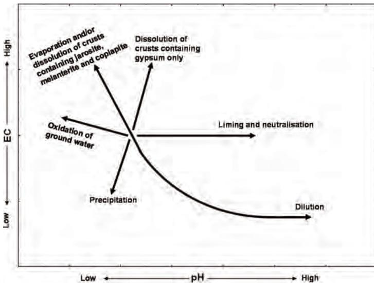
**Figure 2** Geochemical vectors for the evolution of water (Tutu et al.2008)
