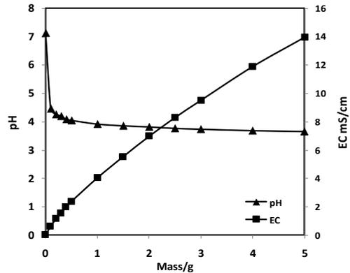
**Figure 1** Potential effect of crusts on receiving waters (dissolution in 100 mL of deionised water)
