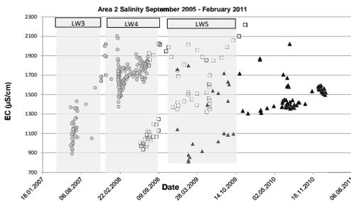
**Figure 5** Evolution of water salinities with extraction of progressive longwalls 3 to 5. Waters present after the cessation of extraction are more saline than those present during longwall extraction.
