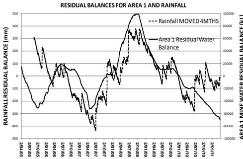
Figure 8 Area 1 rainfall and mine water balance.
