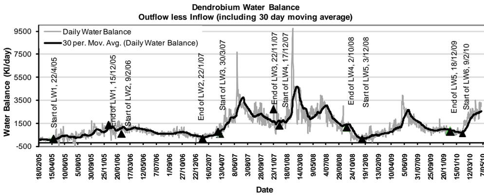
Figure 2 Dendrobium Water Balance through time showing periods of water inflow to the mine.
