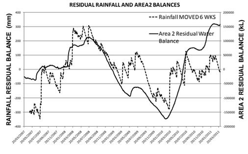
Figure 9 Area 2 rainfall and mine water balance.
