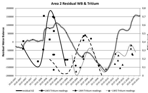
**Figure 6** Residual water balance for Area 2 plotted with Tritium values for the various longwall-lines have been drawn to elucidate the trends in Tritium levels.
