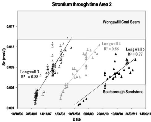
**Figure 4** Variation Sr in goaf waters with time, fields for Scarborough Sandstone and Wongawilli Coal seam are defined by average values  $\pm 1$  Standard deviation.
