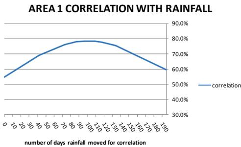
Figure 10 Area 1 correlation of rainfall with mine water balance by moving rainfall forward in time incrementally.
