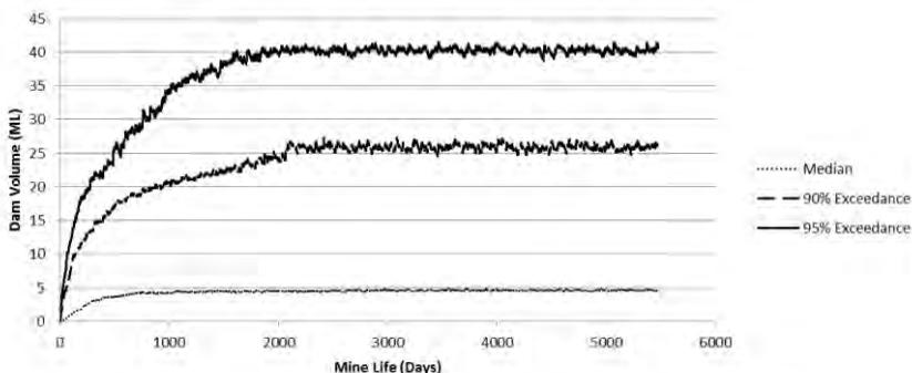
**Figure 1** Results of probabilistic simulation for Dam 1
