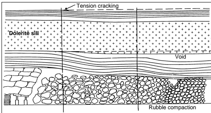
**Figure 4** Cross-section through a high extraction panel illustrating arrested subsidence by a dolerite sill. Note the void that forms at the base of the sill (from Fauconnier and Kersten 1982).
