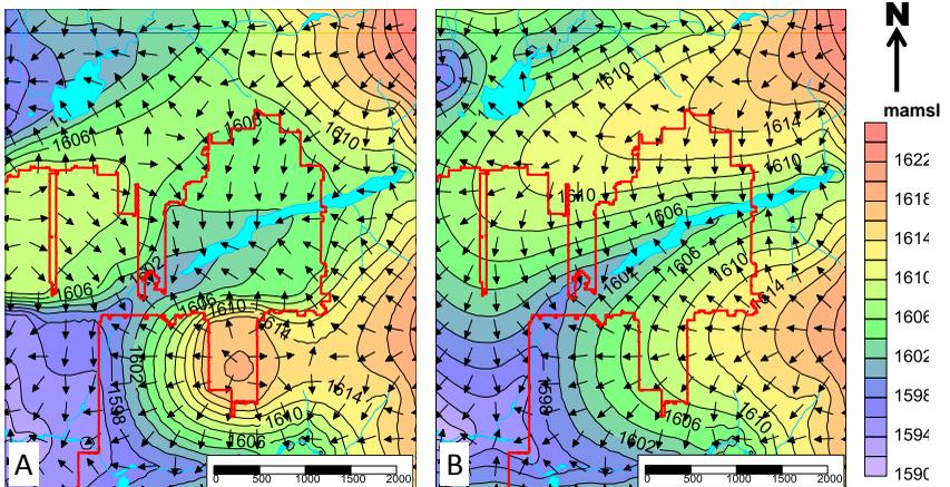
**Figure 3** Modelled changes in pre-mining groundwater level (A) relative to post-mining level (B). Scale bars indicate distance in metres.
