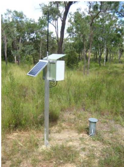
**Figure 5:** *Groundwater bore monitoring station*
