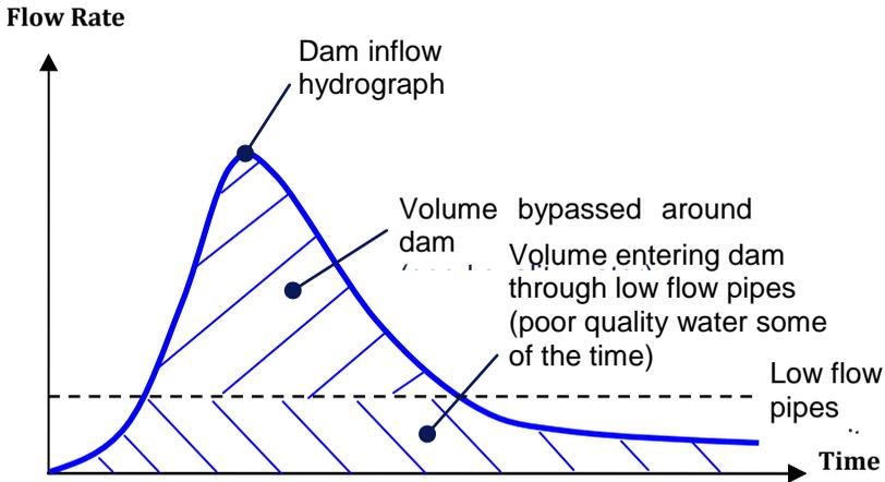
**Figure 4:** Flow-based segregation of good and poor quality water in high flow bypass facility
