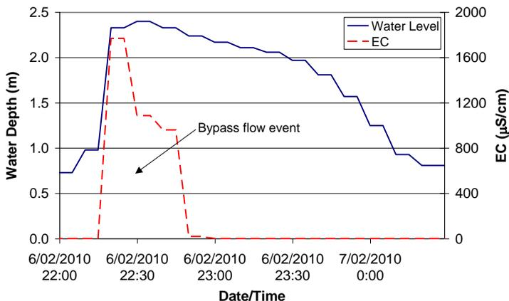
**Figure 8:** Performance of high flow bypass facilities – Settlement Dam
