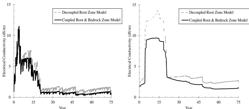
**Figure 3** Sensitivity of the simulated mean root zone salinity (left) and mean deep drainage salinity (right) between the coupled and decoupled modes for the LIC site base case scenario under Buffel Grass (2 ML/ha/yr).
