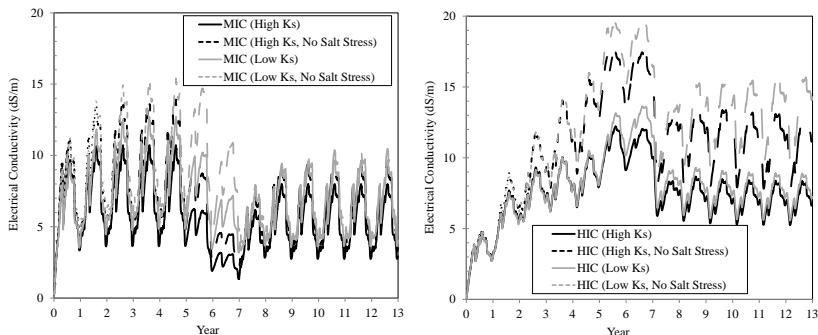
**Figure 5** Sensitivity of the simulated mean root zone salinity to the inclusion of salinity stress and the bedrock  $K_s$  for the MIC (left) and HIC (right) sites under Leucaena (4 ML/ha/yr).
