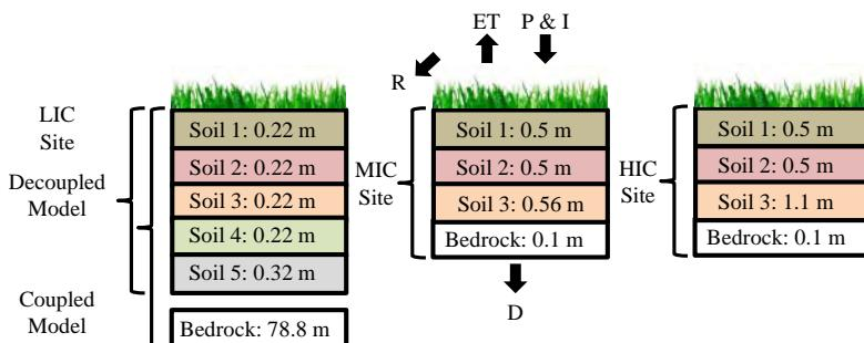
**Figure 1** Conceptual model of the water budget, material layering, and material thicknesses for the three agricultural plots (not to scale).
