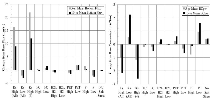
**Figure 2** Sensitivity of the simulated mean deep drainage rate into the bedrock (left) and mean root zone salinity (right) for the LIC site under Leucaena (2 ML/ha/yr) relative to the base case simulation.
