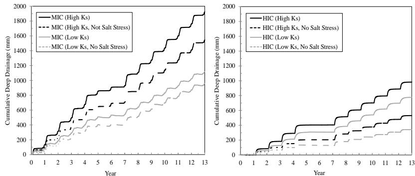
**Figure 4** Sensitivity of the simulated cumulative amount of deep drainage into bedrock to the inclusion of salinity stress and the bedrock  $K_s$  for the MIC (left) and HIC (right) sites under Leucaena (4 ML/ha/yr).
