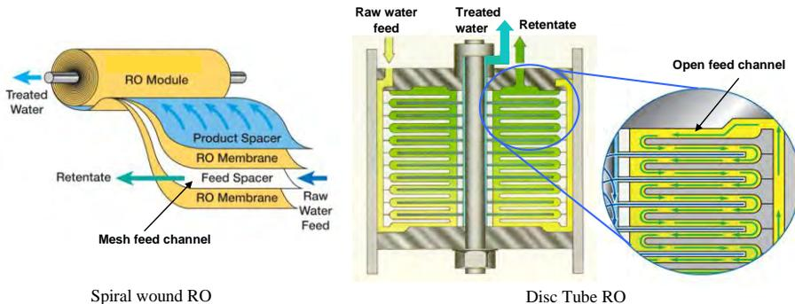
**Figure 3** RO module configurations
