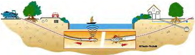
Figure 1 Schematic presentation of horizontal drilling (Tracto-Technik 2010)
